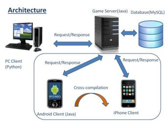
Figure 9. DeBugger Architect including Mobile Debugger. This shows the relationship between a PC Client, Android Client, iPhone Client and the Server
